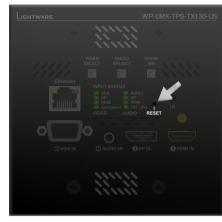
In few cases (after firmware upgrade, etc) you may need to reset the device. Pushing the reset button results the same as you disconnect and reconnect the power adaptor to the transmitter. To reseting the device follow the steps:
