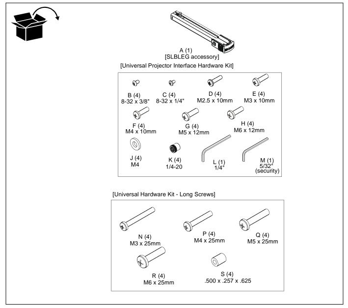
**NOTE:** The SLBLEG is designed to be used as an additional leg along with Chief® SLBU/SLMU interface brackets. The following installation instructions show how to install it simultaneously to the SLBU/SLMU interface bracket. Refer to SLBU/SLMU installation instructions for further installation instructions.
