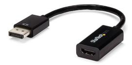
The DP2HD4KS DisplayPort to HDMI adapter enables you to connect a DisplayPort-equipped desktop or laptop computer, such as the HP EliteBook 8570p / 8470p, to an HDMI display. This adapter is compatible with DisplayPort 1.2 & HDMI 4K @ 30 Hz and as a result can support video resolutions up to Ultra HD (4K) as well as the accompanying digital audio up to 7.1 channel surround sound.
