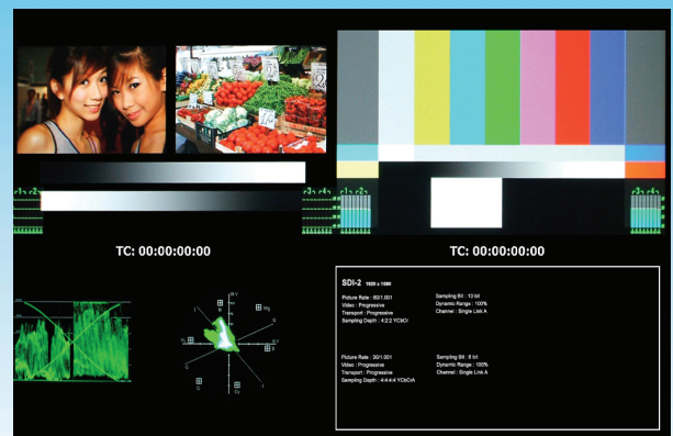
Dual Display Mode with Waveform & Vector
