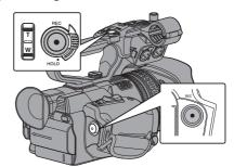
Press the [REC] button to start recording to the SD card.
