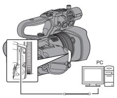
2 Select [Change] using the cross-shaped button (▲▼), and press the Set button (●). The camera recorder switches to USB mode.
