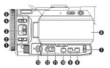
1 [FULL AUTO] Full Auto Selection Button Press and hold the button to switch the Full Auto mode ON and OFF. Full Auto mode adjusts the Iris, Gain, Shutter and White Balance automatically.
