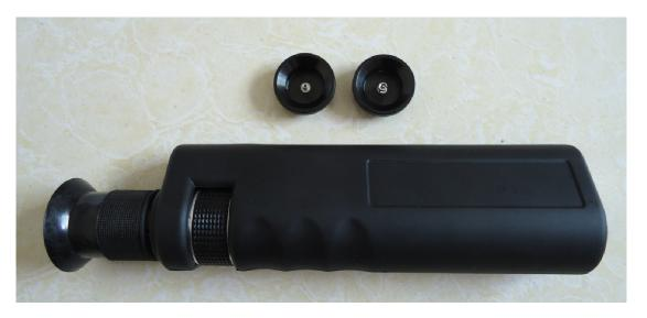
• The YW-400XA fiber optic microscope utilizes a white light LED for coaxial illumination .Light is introduced into the optical path (axis) so that it comes out the tip of the objective lens and strikes the ferrule perpendicular to the end face .This method of illumination produces a high level of resolution providing excellent detail of scratches and contamination.
