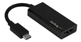
This USB-C to HDMI adapter lets you output HDMI video and audio from a USB Type-C device, such as a USB-C equipped MacBook, with support for Ultra HD 4K at 60 Hz. This adapter works with USB-C devices that pass a DisplayPort video signal, and it's also compatible with Thunderbolt 3 ports.
