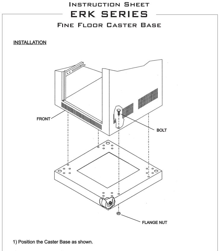
2) Install the bolts and flange nuts, then tighten.
