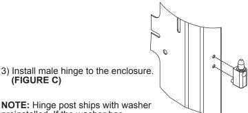
**NOTE:** Hinge post ships with washer preinstalled. If the washer has come off during shipping, it must be reinstalled.
