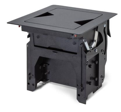
The Table Connect Box (TBC) is a cable pass-through bracket for six AV signal cables, for easy BYOD connection, which also hosts two power outlets. An extender for video signals can be mounted under desk and the cables can be connected, without being visible when not in use.
