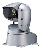
The new AW-HR140 is an integrated remote camera system that incorporates an outdoor housing, camera, lens and pantilt head.
