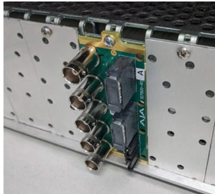
Figure 8. Rear Card Inserted Into Frame Seating Slot
