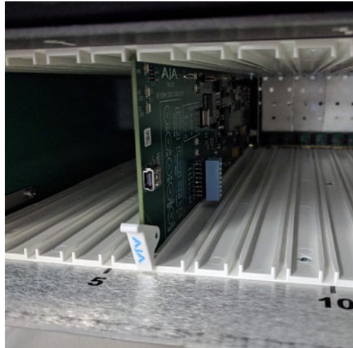
Figure 9. OG-UDC card inserted Into Right Slot
