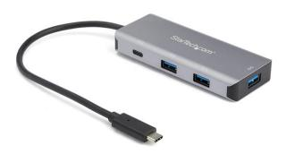
Expand the connectivity of your USB-C laptop withthisnew generation USB-CGen 2huboffering 10Gbpssupporting greater bandwidth to connected devices and fasterdata transferspeeds. Thisbus-powered4-PortUSB-Chubplugsinto the USB Type-C or Thunderbolt 3 port on your device, addingone USB-C port and three USB-A ports, so you can quickly connect more USB devices.
