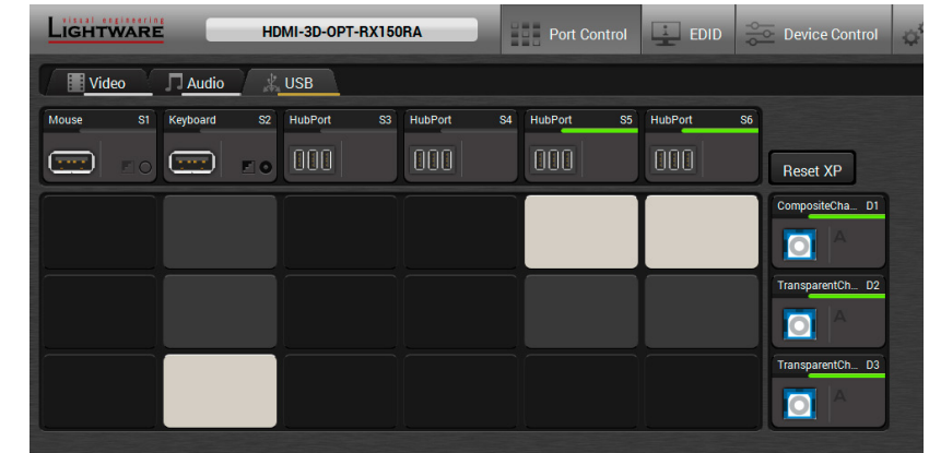
USB KVM layer in case of a connected 4-port USB HUB
