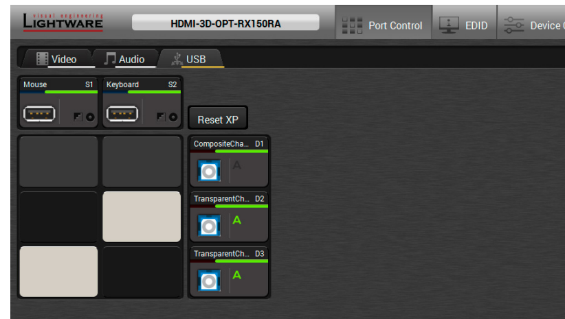
USB KVM layer in the Receiver
