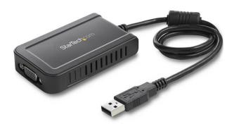
The USB2VGAE3 USB VGA Multi-Monitor External Video Adapter lets you add a high-resolution (1920x1200) external VGA output to your desktop or laptop computer, using an available USB 2.0 port.
